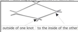
Knot to knot (bar measure) is the length of the full bar measured from the outside of one knot to the inside of the other.
